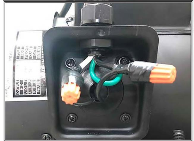
Figure 62. W1862 motor junction box.
