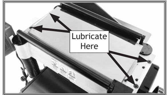
Figure 35. Lubrication locations for feed roller bushings.
