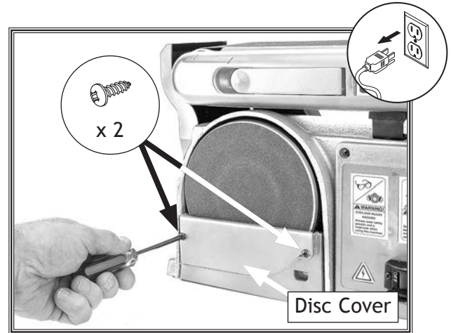
Figure 22. Removing disc cover.
