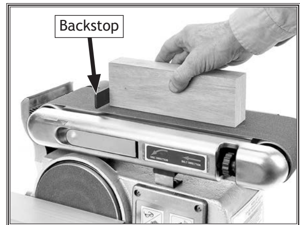
Figure 18. Horizontal belt sanding.
