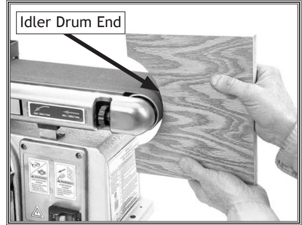
Figure 19. Sanding an inside curve.
