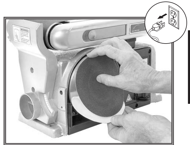
Figure 23. Installing sanding disc.
