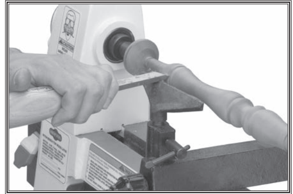
Figure 38. Example of typical spindle turning operation.
