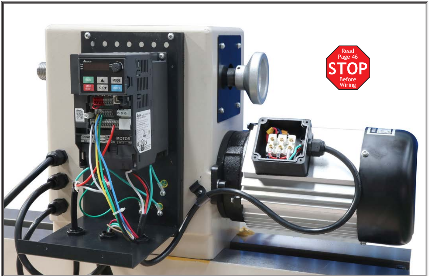
Figure 51. Inverter box and motor box locations.
