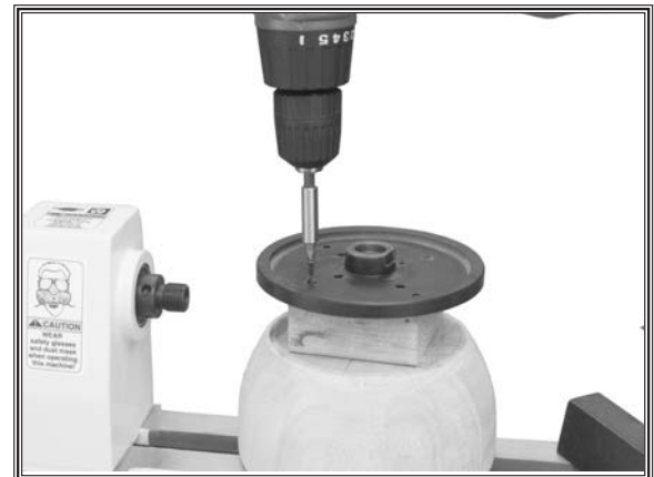
Figure 43. Example of attaching faceplate to workpiece.
