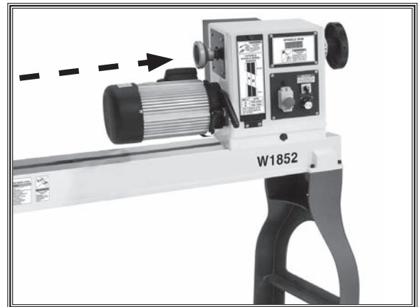
Figure 45. Example of lathe prepared for outboard turning.
