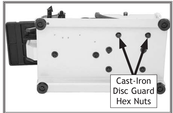
Figure 36. Location of cast-iron disc guard hex nuts.
