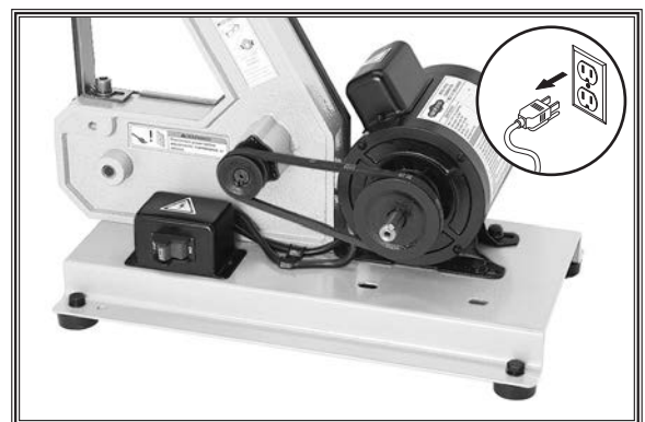
Figure 37. New V-belt installed.
