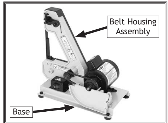
Figure 9. Belt housing assembly installed.
