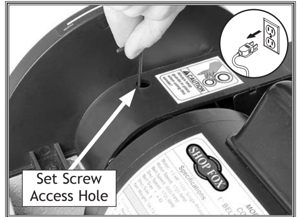
Figure 31. Location of access hole for sanding disc set screw.
