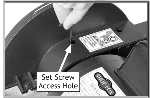
Figure 14. Securing sanding disc set screw.
