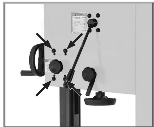
Figure 96. Guide post adjustment cap screws.
