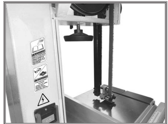
Figure 98. Guide post guard removed.
