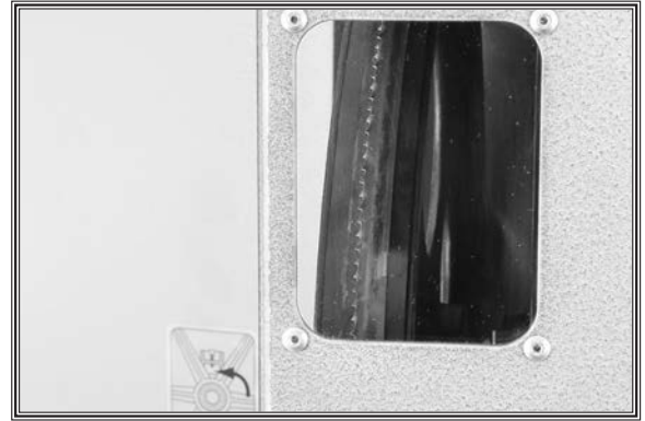
Figure 42. View of blade through tracking window.
