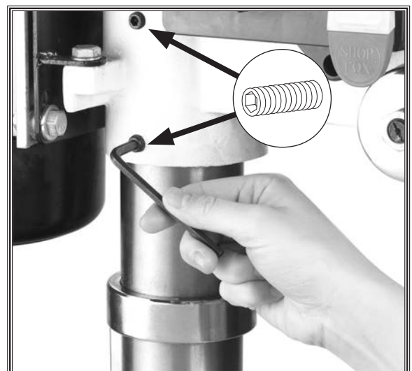
Figure 23. Securing the headstock to the column.
