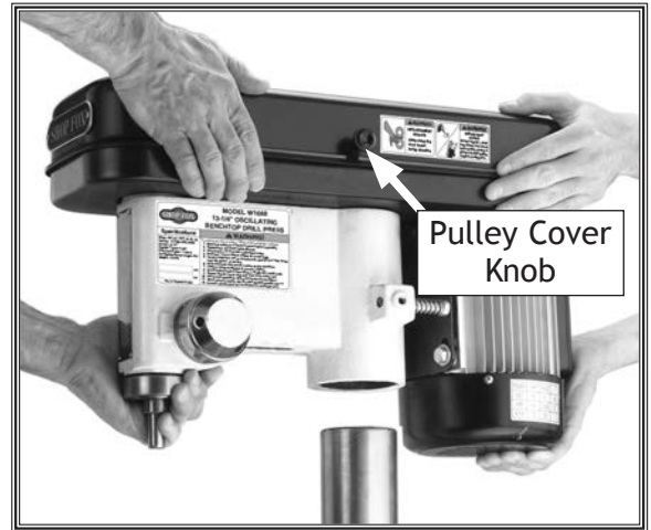
Figure 21. Aligning the pocket in the headstock with the column.
