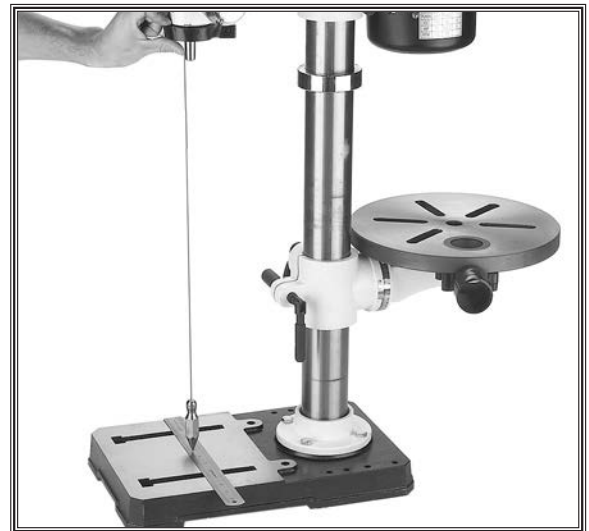
Figure 22. Aligning headstock with base (W1668 shown).
