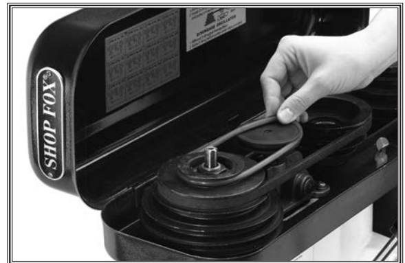
Figure 48. Stretching belt to fit on pulleys.
