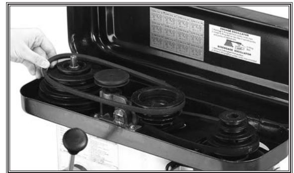
Figure 37. Adjusting belt to desired speed.
