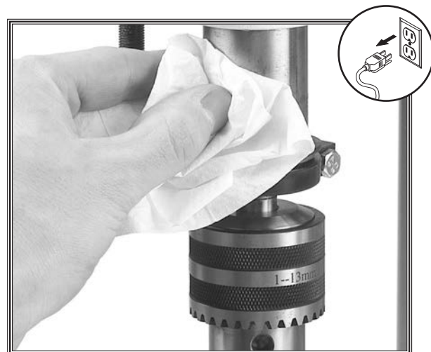
Figure 53. Cleaning quill surfaces.
