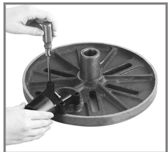
Figure 14. Installing the dust port.
