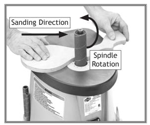
Figure 13. Sanding workpiece.
