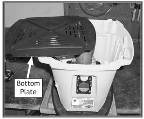
**Figure 17.** Sander turned upside down with bottom plate removed.
