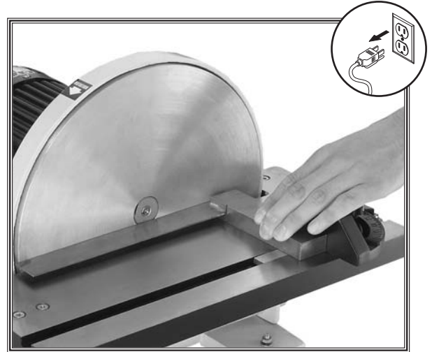
Figure 20. Squaring miter gauge to disc.
