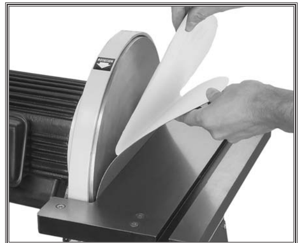
Figure 15. Removing the paper backing.
