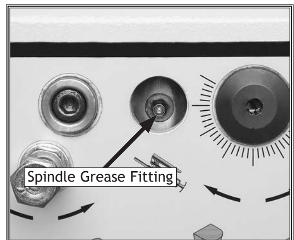
Figure 47. Spindle grease fitting.
