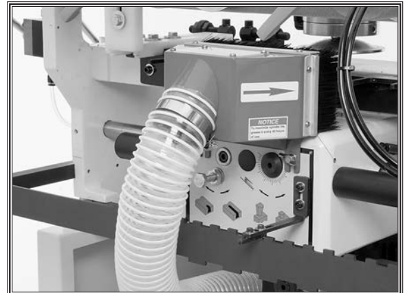
Figure 8. Dust hose attached to guard.
