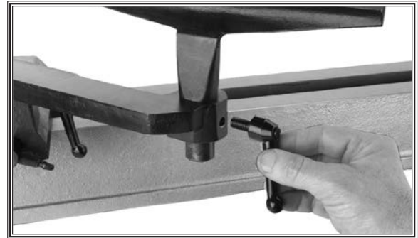
Figure 9. Installing tool rest handle.
