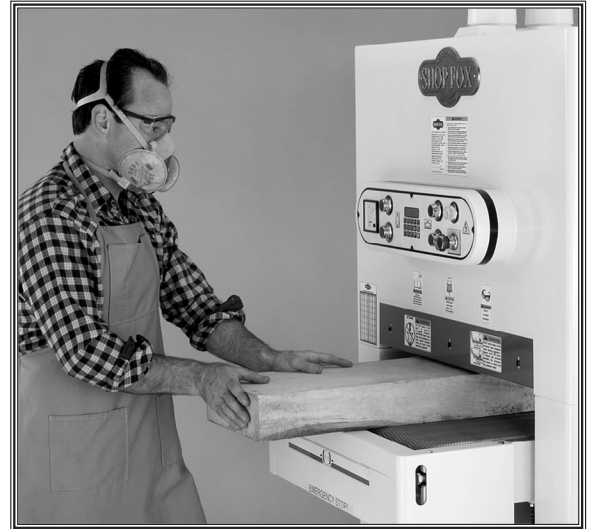
Figure 21. Operator feeding workpiece at correct body position and out of the way of potential kickback.
