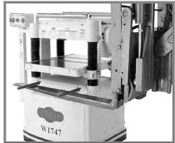
Figure 4. Example of planer being lifted using forklift.
