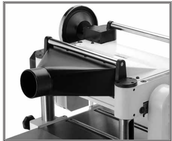
Figure 8. Dust hood installed.
