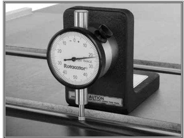
Figure 19. Rotacator measuring table roller protrusion.
