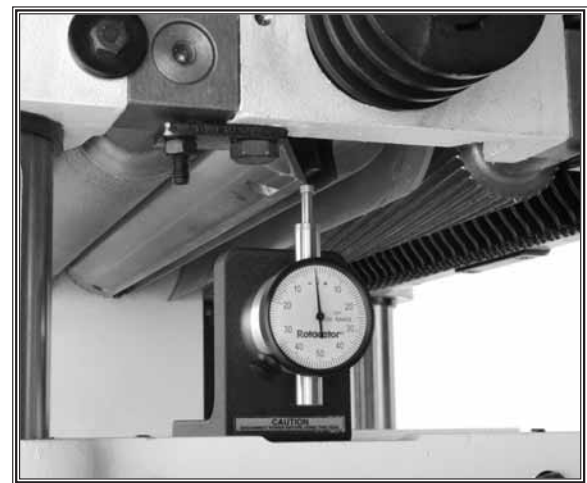
Figure 38. Finding BDC of cutterhead.
