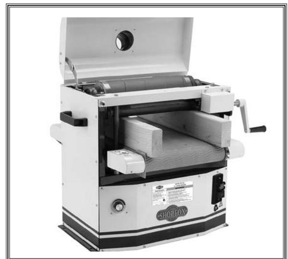
**Figure 28.** Gauge boards in position.
