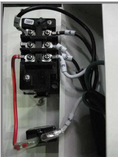
Figure 67. ON/OFF switch wiring.
