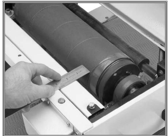
**Figure 31.** Measuring drum alignment.
