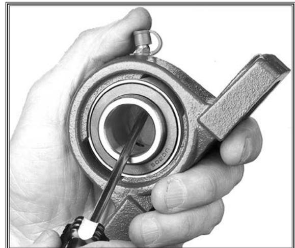
Figure 59. Bearing positioning for removal.
