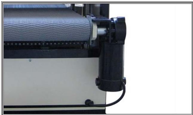
Figure 63. Feed motor.
