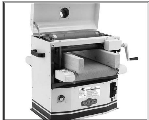
**Figure 38.** Gauge boards in position.
