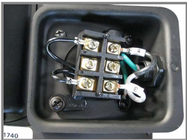
Figure 64. Drum motor wiring.
