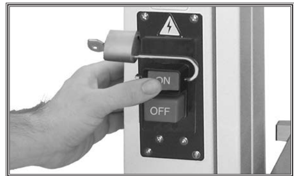
Figure 27. Switch disabling padlock inserted into ON button.
