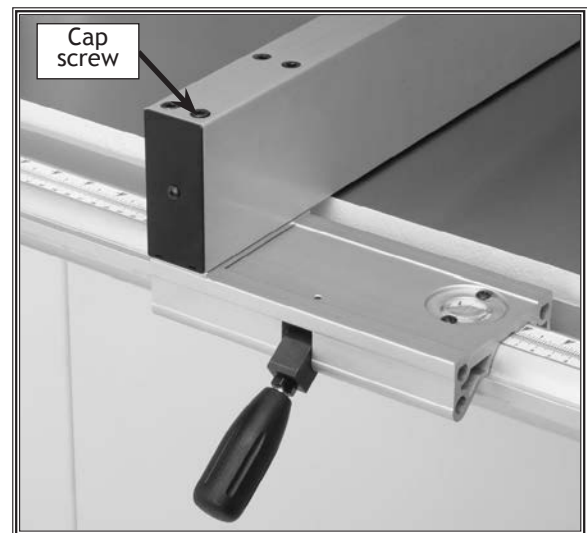
Figure 20. Adjusting the fence parallelism.
