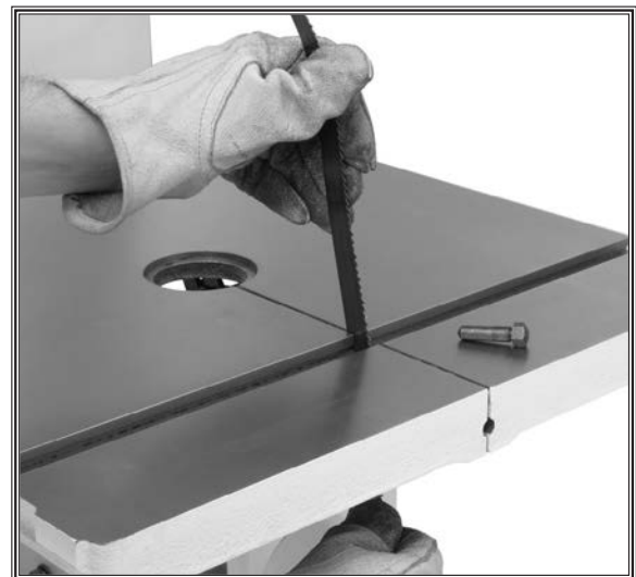
Figure 33. Sliding the blade through table slot.
