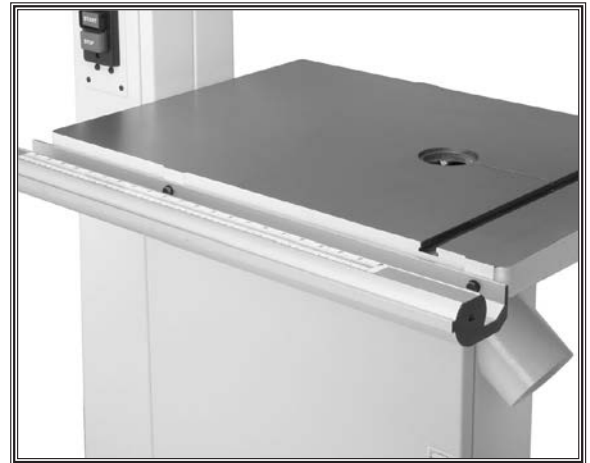
Figure 13. Table and large rail positioning.
