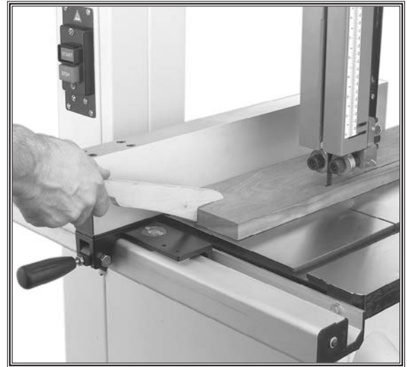
Figure 38. Safely ripping a board.
