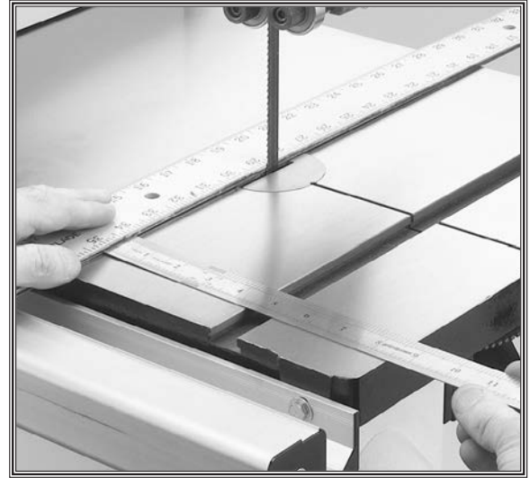
Figure 18. Squaring the miter slot to blade.
