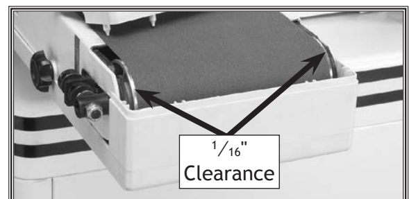
Figure 25. Proper belt tracking (guard removed for clarity).
