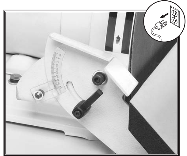
Figure 12. Table tilt set at 45°.
