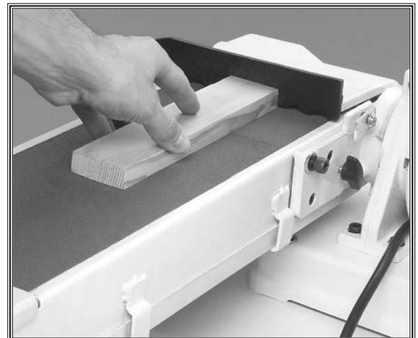
Figure 17. Flat sanding operation.
