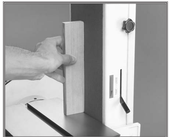
Figure 14. Flat sanding operation.
