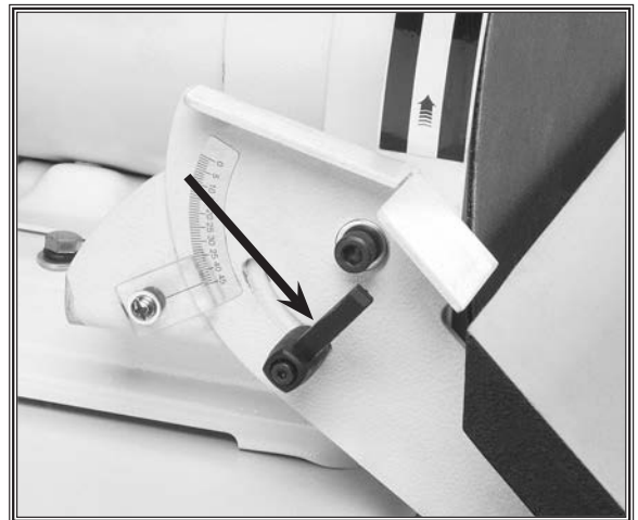
Figure 8. Installed tilting knobs.
