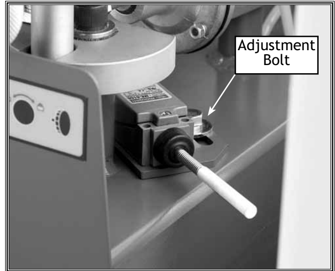
Figure 17. Tracking safety switch adj. bolt.
