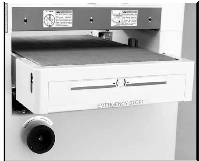
Figure 31. Emergency stop plate.
