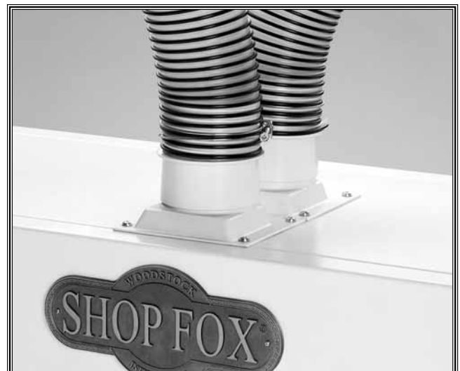
Figure 11. Dust collection hose attached to dust port.
