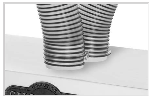
Figure 3. Dust collection hoses attached to dust ports.
