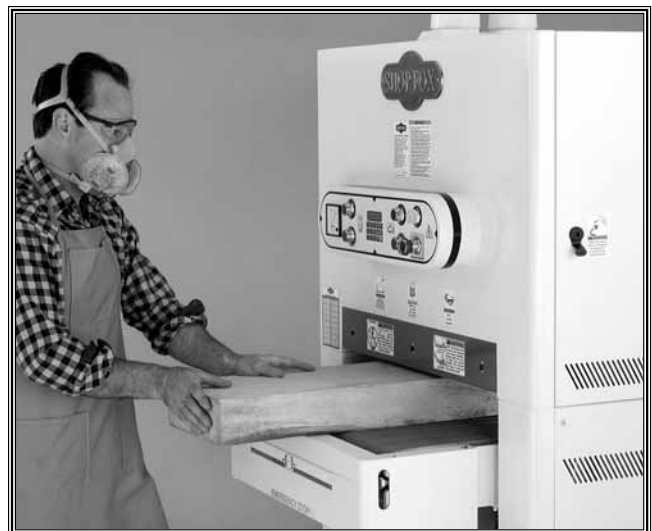
Figure 34. Operator feeding workpiece in correct body position and out of the way of potential kickback.
