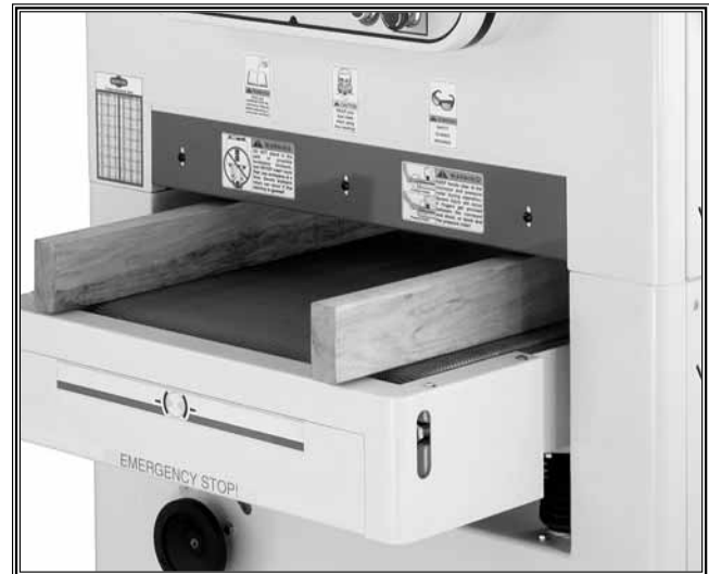
Figure 21. Gauge boards placed under pressure rollers as a gauge.
