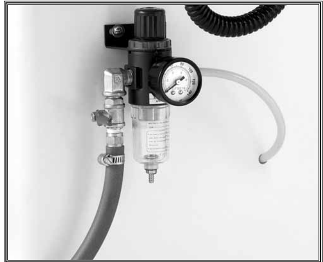
Figure 6. Air hose attached to regulator.
