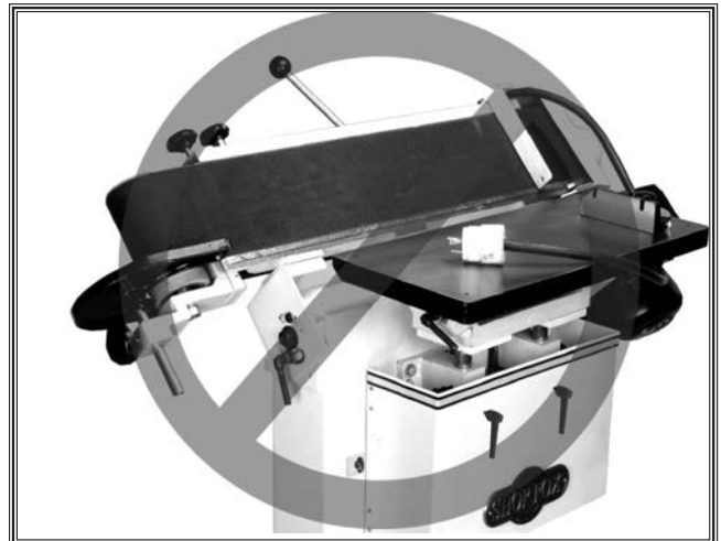
Figure 45. Incorrect platen tilted position.
