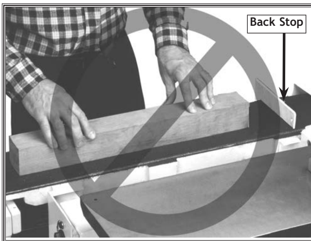
Figure 51. Incorrect face sanding away from back stop.
