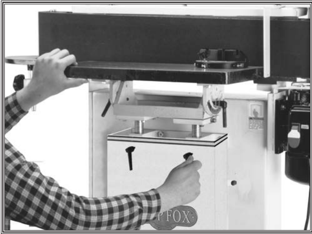
Figure 36. Hold the main table and loosen the lock lever.
