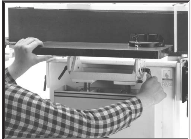
Figure 38. Hold the main table and loosen the lock lever.
