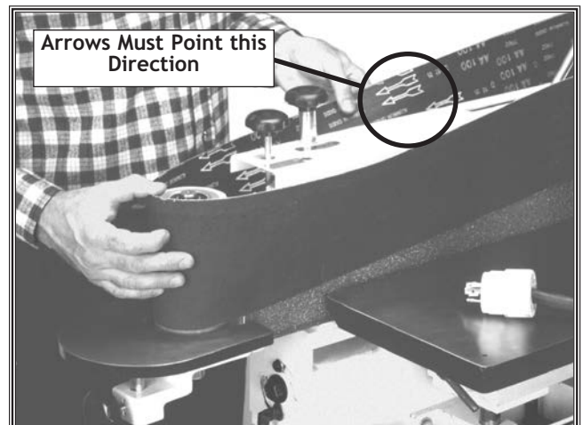
Figure 22. Sanding belt directional installation.
