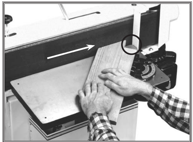
Figure 49. ALWAYS sand wood with sharp corners at the trailing-edge of the sanding operation.
