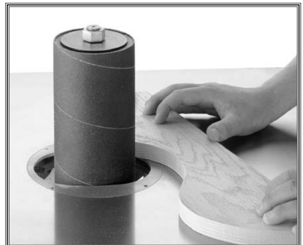
Figure 28. Spindle sanding example.
