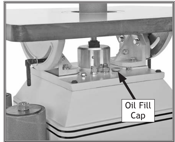
Figure 31. Oil fill cap location.
