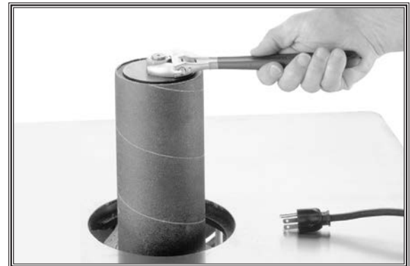
Figure 24. Removing sanding sleeve.
