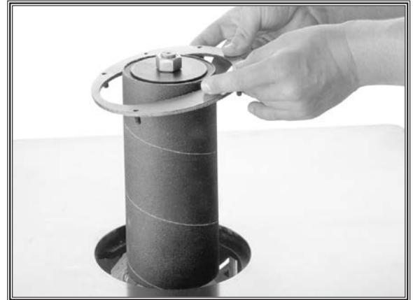
Figure 26. Installing table insert.
