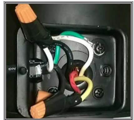
Figure 35. Motor wiring 120V.
