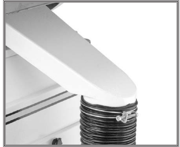
Figure 18. Dust port connected to dust collection system.
