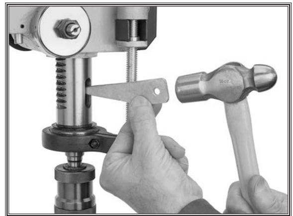
Figure 26. Example of using drift key to remove arbor from spindle.
