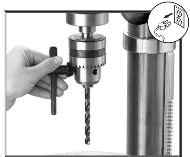
Figure 27. Example of tightening chuck with chuck key.
