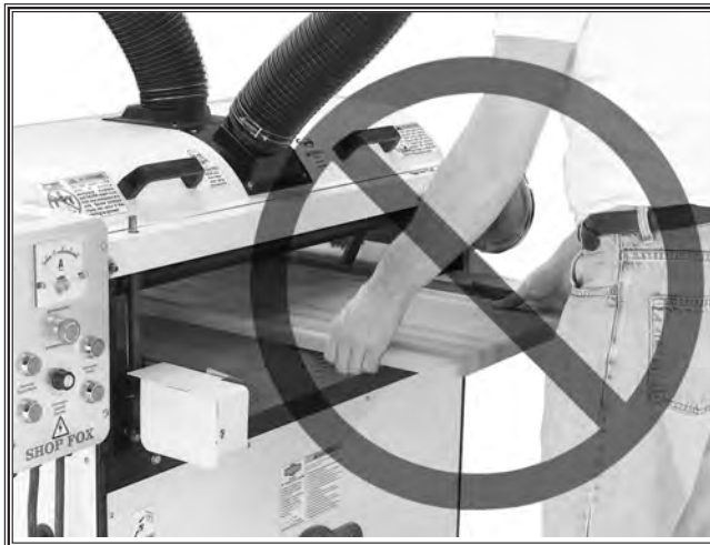
Figure 47. DO NOT stand in the path of where the workpiece could be projected.
