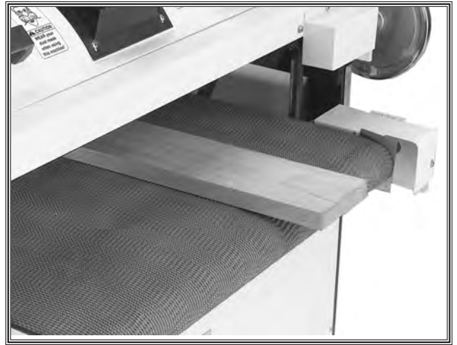
Figure 8. ALWAYS sand the workpiece with it sitting flat against the conveyor belt.
