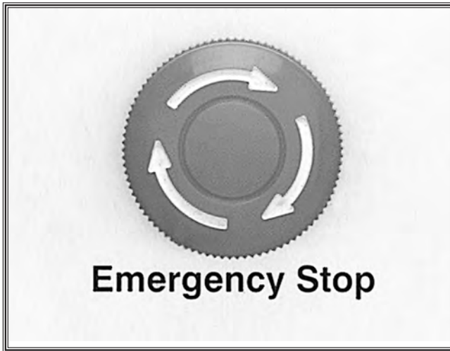
Figure 46. Main power ON/OFF safety switch.
