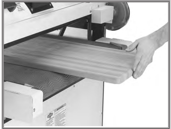
Figure 2. ALWAYS keep fingers away from conveyor and the underside of the stock.
