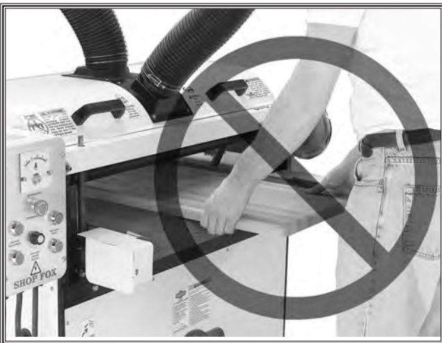
Figure 3. NEVER stand in the path of potential workpiece kickback.
