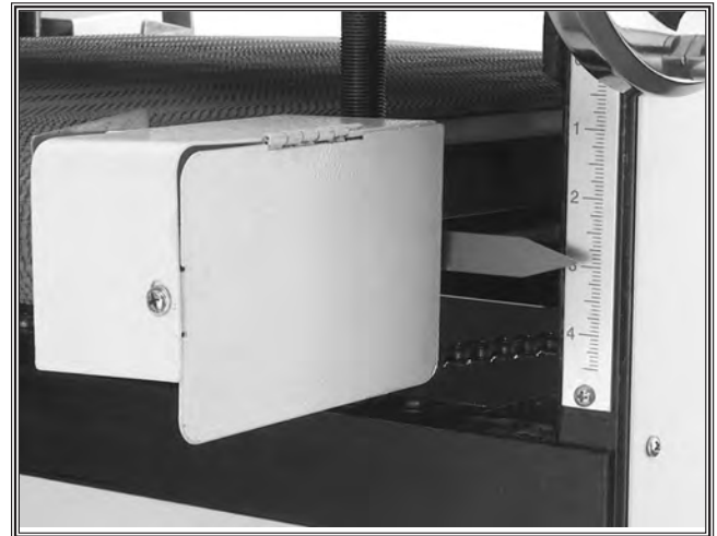
Figure 44. Depth scale indicates depth of cut.
