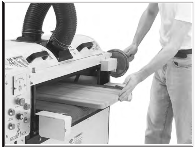
Figure 49. ALWAYS stand out of the way of where the workpiece could be projected, and keep fingers away from the underside of the workpiece.
