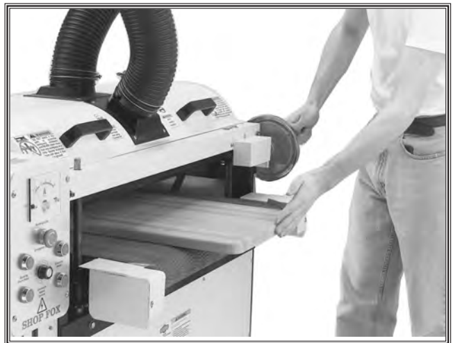
Figure 4. ALWAYS keep yourself and bystanders away from the path of potential workpiece kickback.
