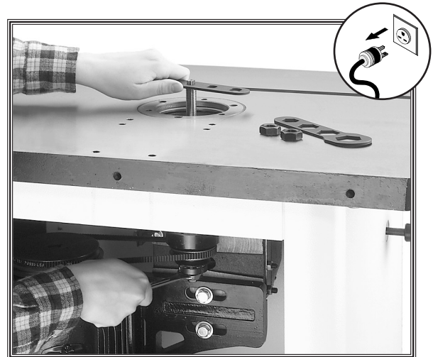
Figure 38. Tightening the drawbar nut.
