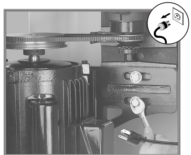
Figure 33. Loosening the motor mount hex bolts.
