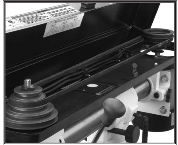
Figure 38. Belt safety cover opened.
