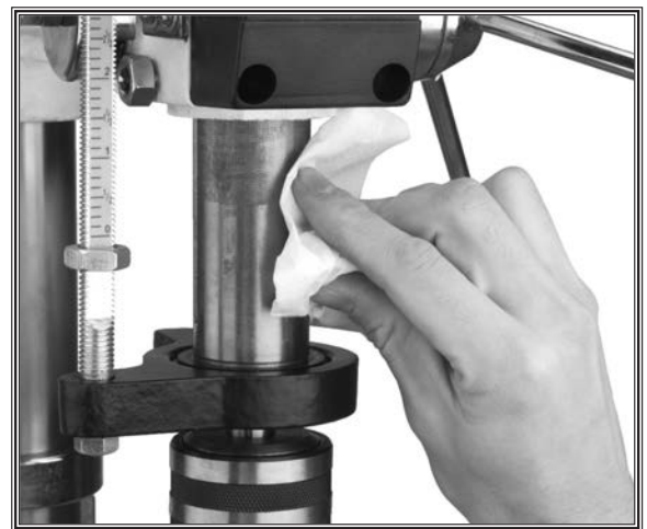
Figure 45. Clean and oil quill shaft.
