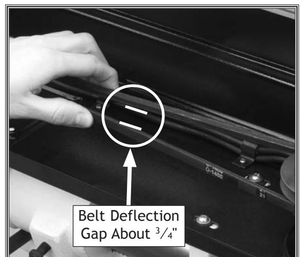
Figure 40. Measuring belt deflection.
