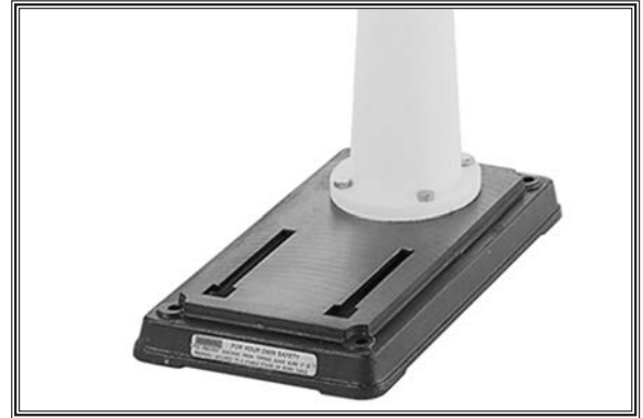
Figure 11. Column secured to base.
