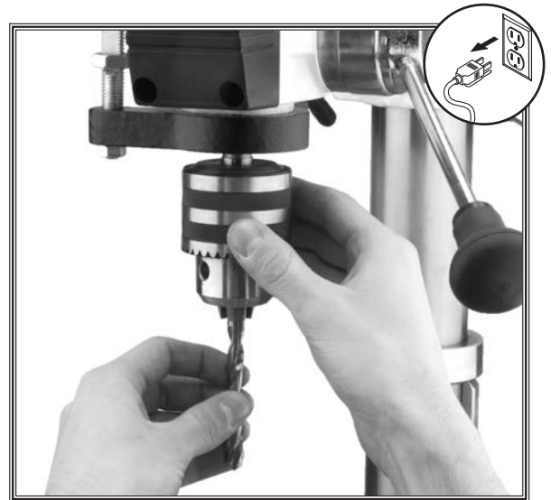
Figure 29. Installing a drill bit.
