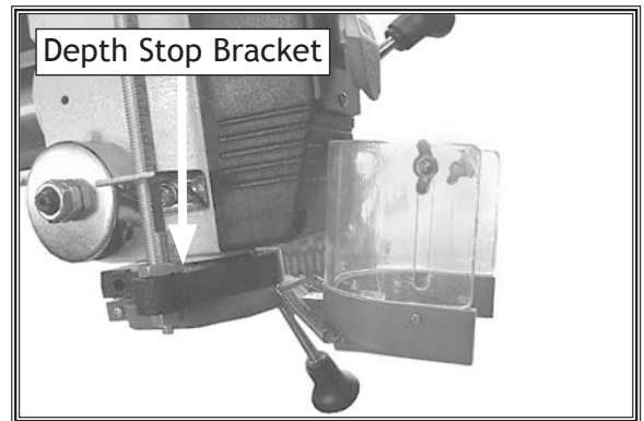
Figure 22. Chuck guard installed on depth stop bracket.
