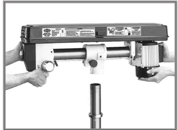
Figure 19. Installing the headstock onto the column.
