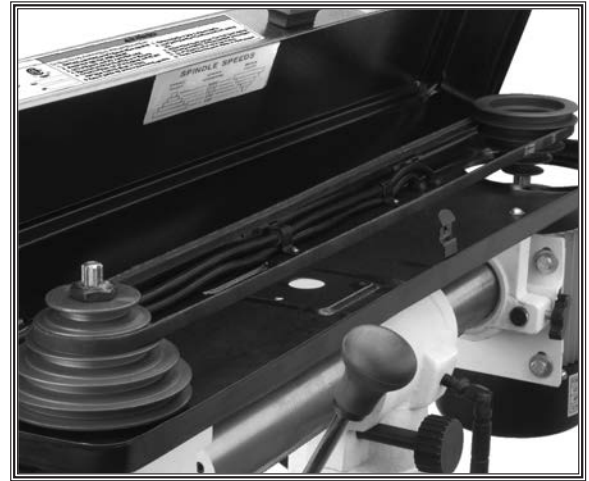
Figure 38. Belt safety cover opened.
