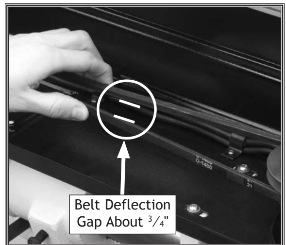
Figure 40. Measuring belt deflection.
