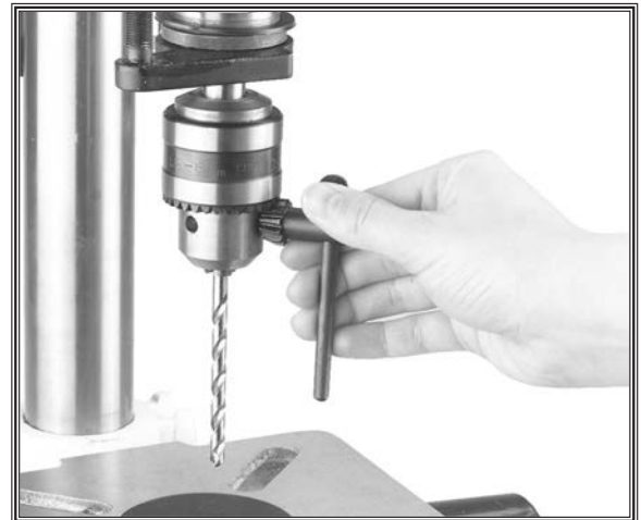
Figure 28. Chuck key engaged (chuck guard removed for clarity).
