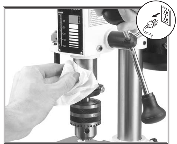
Figure 38. Cleaning quill surfaces.
