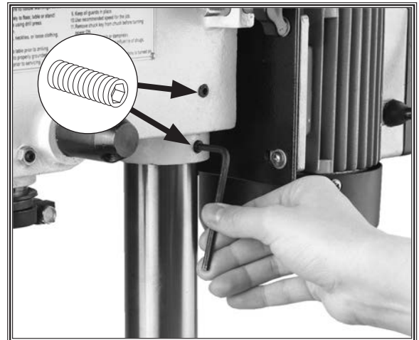
Figure 14. Example of securing headstock to column.
