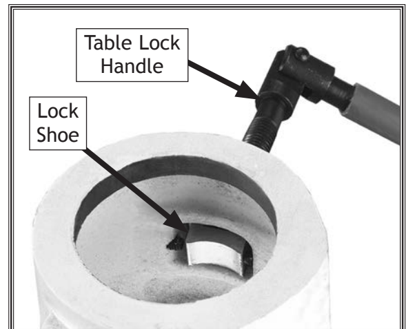
Figure 12. Table lock handle and lock shoe installed in table support bracket.
