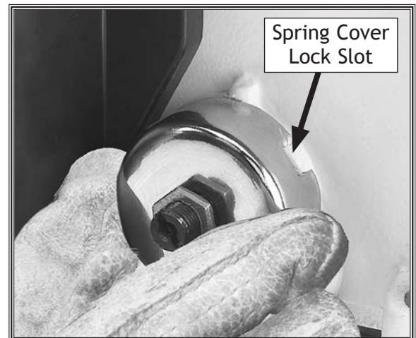
Figure 46. Location of spring cover lock slot.
