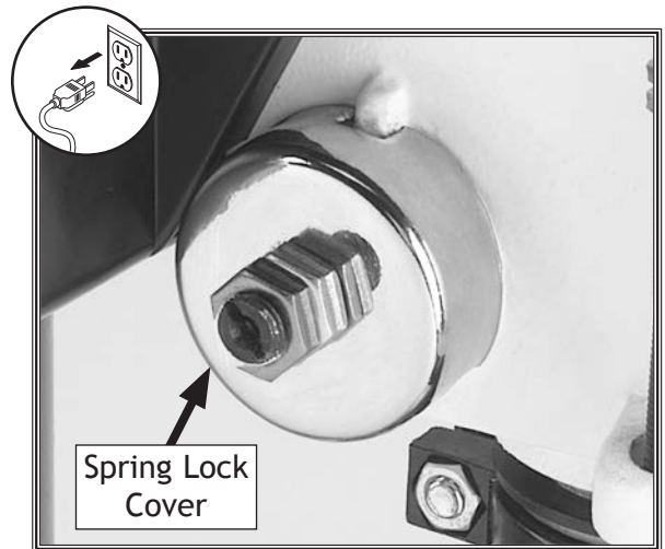
Figure 43. Location of spring lock cover.
