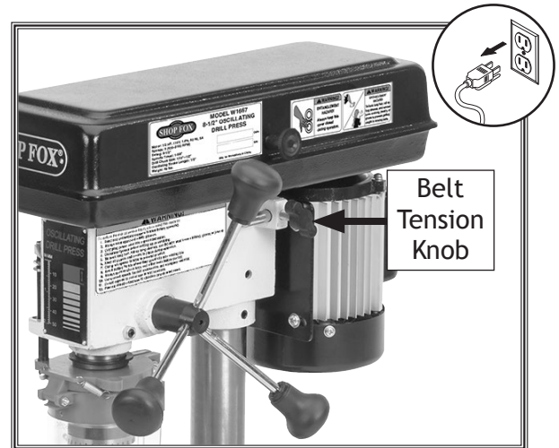
Figure 23. Location of belt tension knob.
