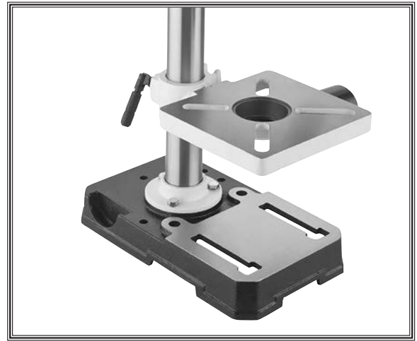
Figure 13. Table installed on column.
