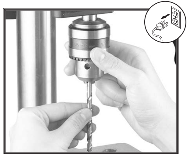
Figure 27. Installing bit (chuck guard removed for clarity).
