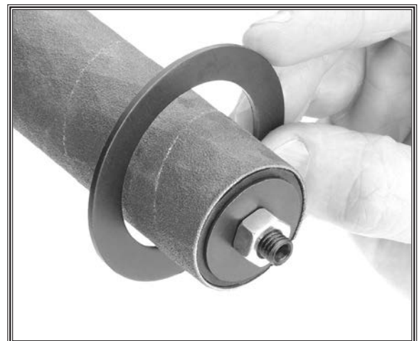
Figure 29. Table insert \frac{1}{4} " bigger than sanding drum.
