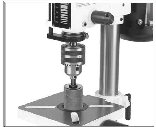
Figure 36. Sanding drum installed and table adjusted.
