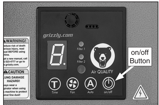
Figure 9. Location of on/off button on control panel.
