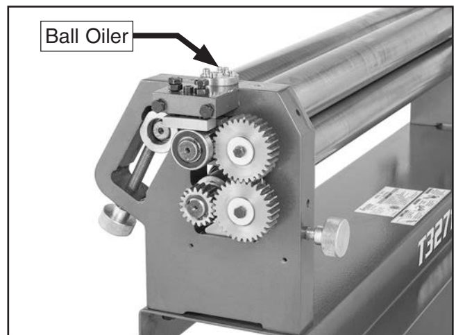
Figure 67. Location of ball oiler.
