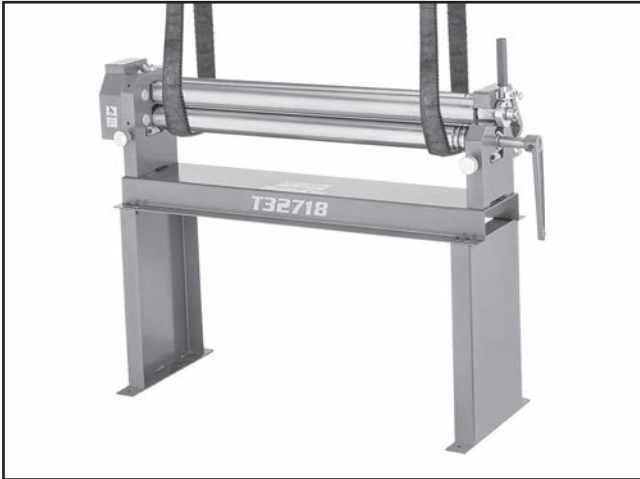
Figure 8. Machine lifted onto legs.
