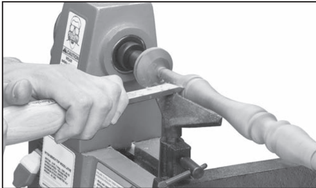
Figure 21. Example of typical spindle turning operation.
