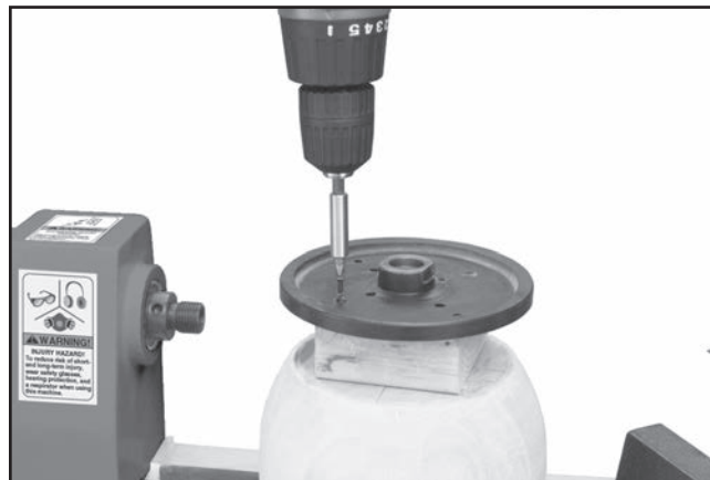
Figure 26. Example of attaching faceplate to workpiece.
