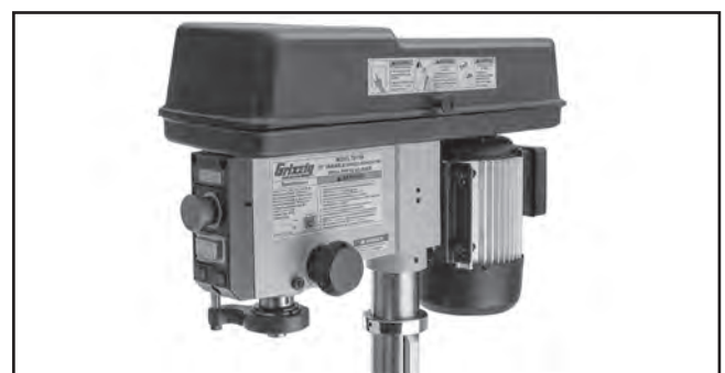
Figure 10. Headstock placed on column.
