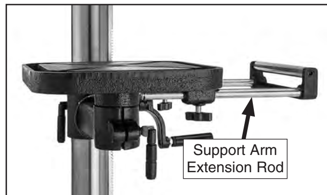
Figure 44. Support arm rod location.
