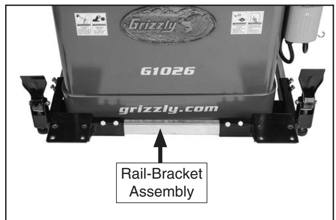
Figure 15. Rail-bracket assembly placed under front of machine.
