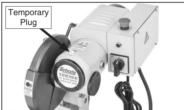
Figure 14. Location of temporary plug.
