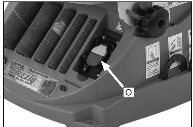
Figure 5. Location ON/OFF paddle switch.
