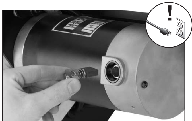
Figure 57. Removing brush from motor.
