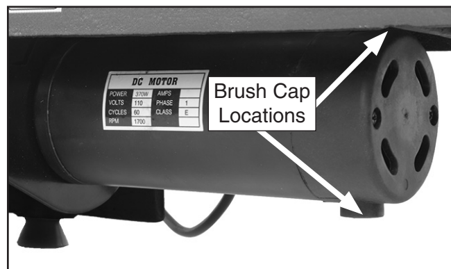
Figure 56. Motor brush cap locations.
