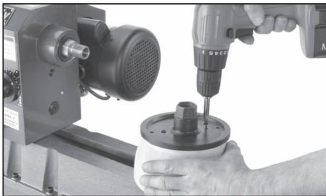
Figure 38. Typical attachment of faceplate to workpiece.
