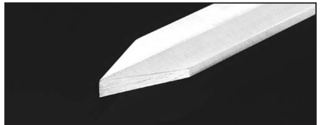
Figure 32. Example of a parting tool.
