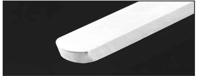
Figure 28. Example of a round nose scraper.
