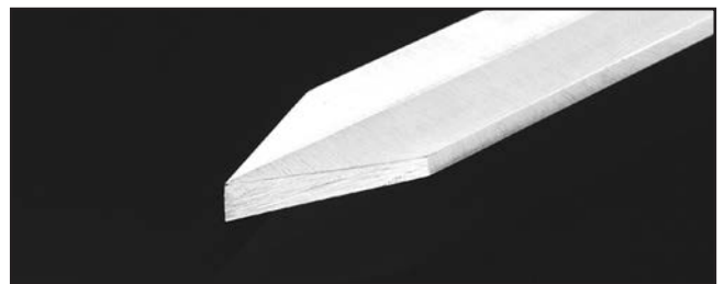
Figure 29. Example of a parting tool.
