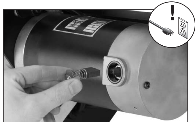
Figure 54. Removing brush from motor.
