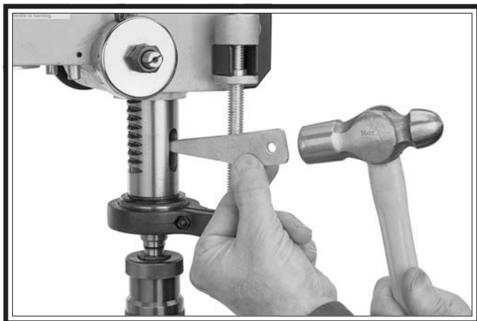
Figure 27. Example of using drift key to remove arbor from spindle.
