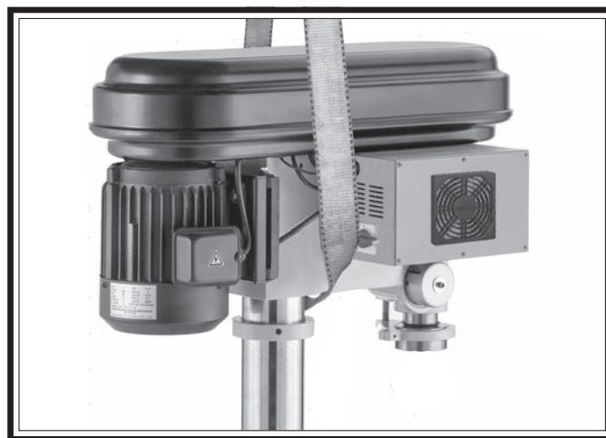
Figure 13. Lifting sling properly placed around headstock.
