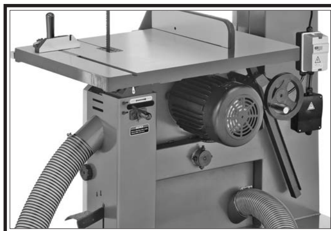
Figure 23. Dust hoses attached.
