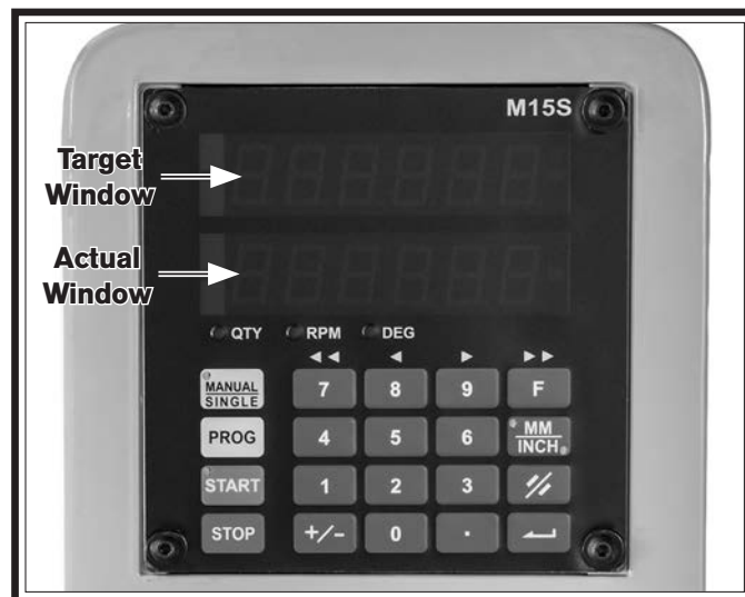
Figure 31. Digital readout windows and keypad.
