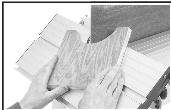
Figure 51. Bevel contour sanding operation example.
