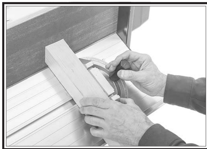
Figure 50. Bevel sanding operation example.
