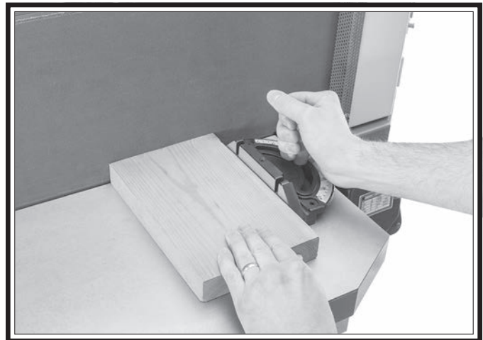
Figure 48. Typical end sanding operation.
