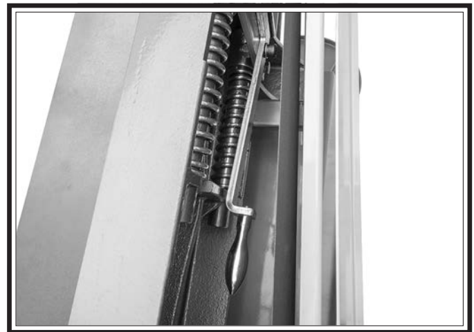
Figure 32. Sanding belt installed and tensioned.
