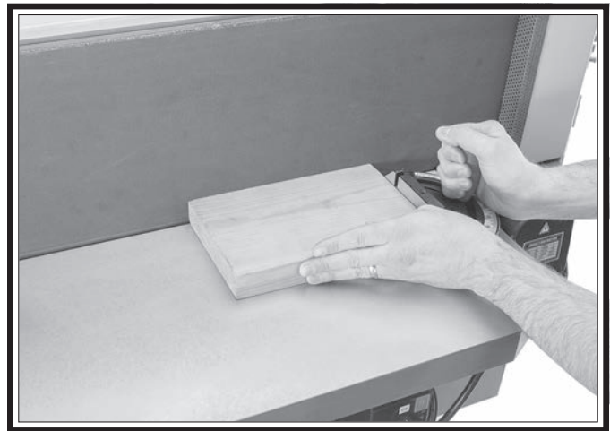
Figure 47. Typical edge sanding operation.
