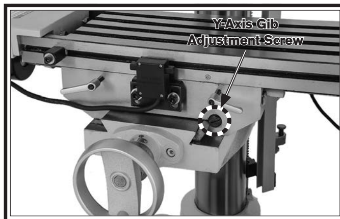
Figure 98. Y-axis gib adjustment screw (1 of 2).
