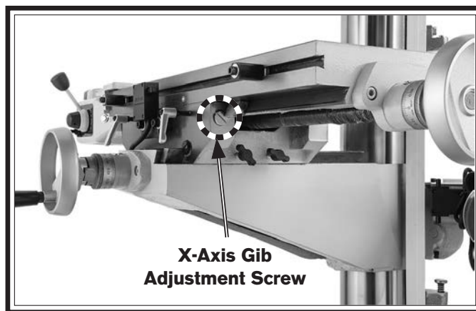
Figure 97. X-axis gib adjustment screw (1 of 2).
