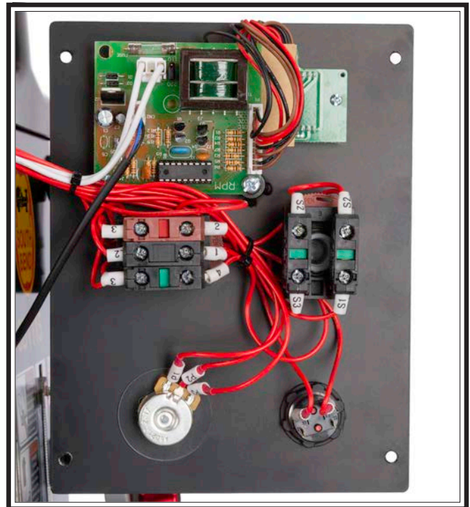
Figure 111. Control panel wiring.
