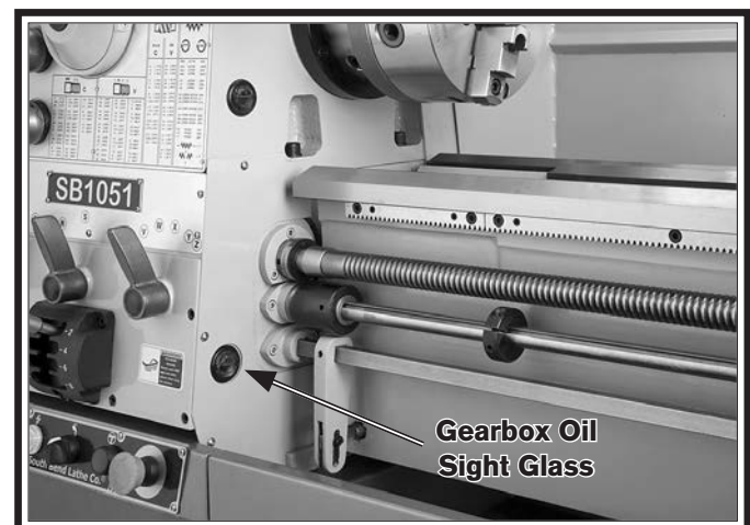
Figure 102. Location of quick-change gearbox oil sight glass.
