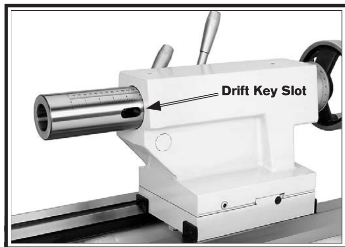
Figure 49. Example photo of the drift key slot in the side of the quill.
