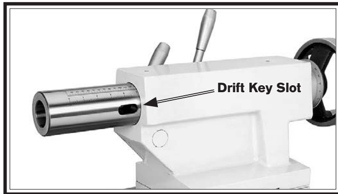
Figure 39. Example photo of the drift key slot in the side of the quill.
