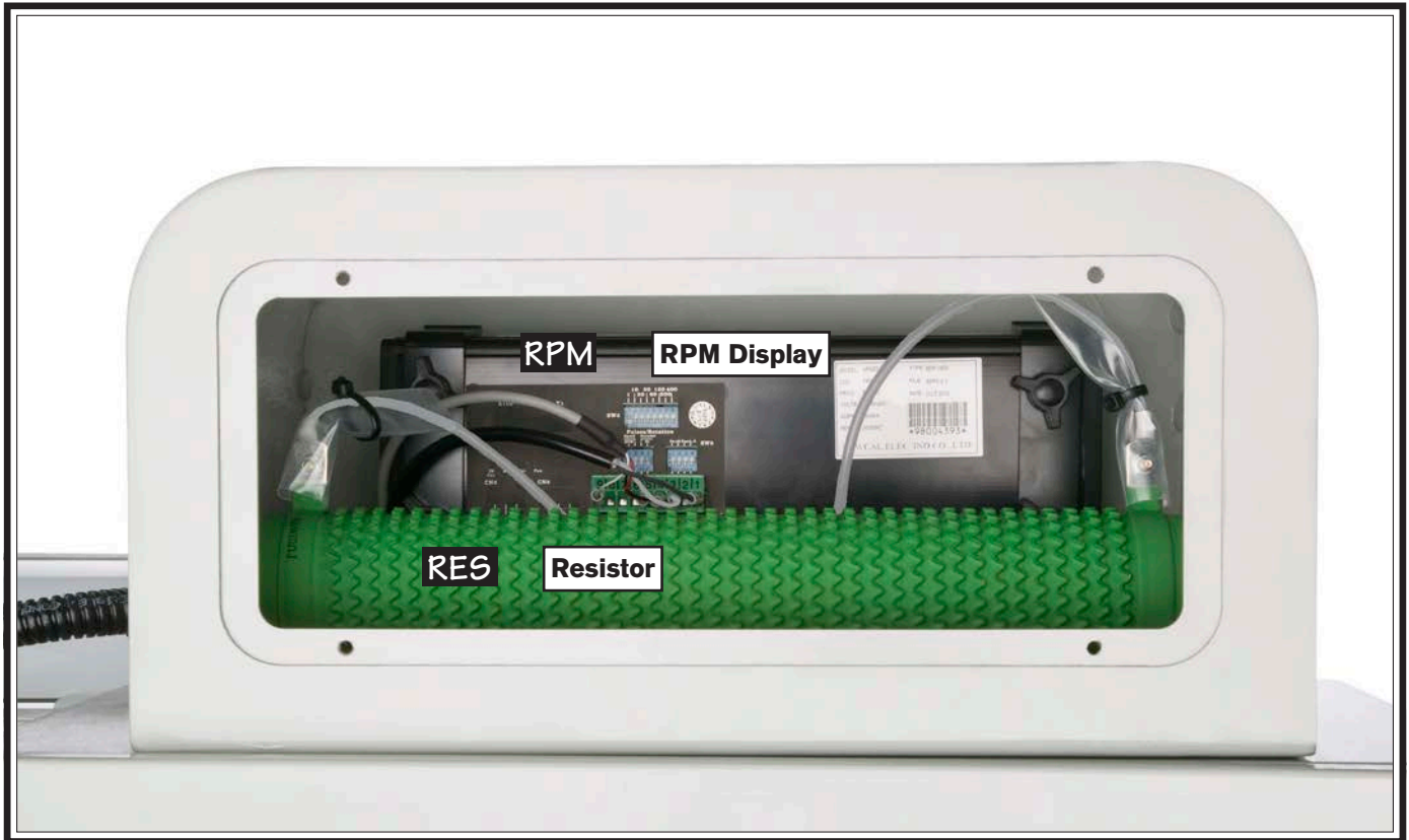
Figure 13. RPM cabinet components and wiring.
