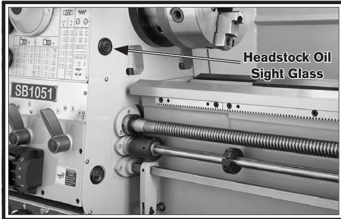
Figure 98. Location of the headstock oil sight glass.
