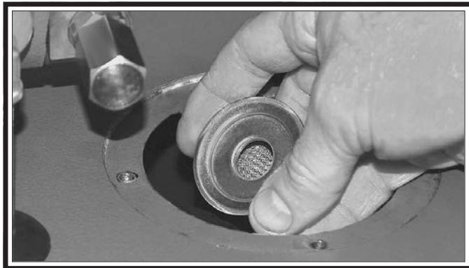
Figure 101. Suction pipe filter screen.
