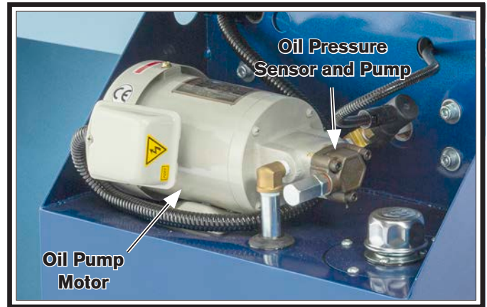
Figure 18. Oil pump motor & pressure sensor.
