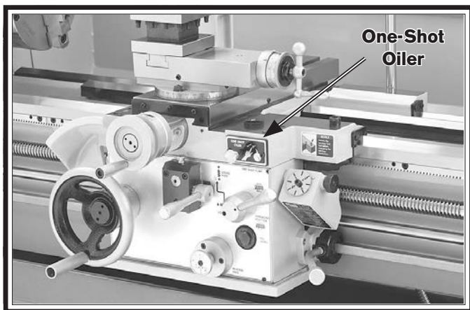
Figure 107. Location of one-shot oiler on the apron.
