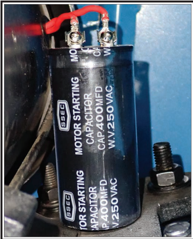
Figure 69. Start Capacitor 400MFD 250VAC.
