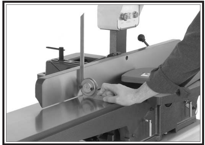
Figure 55. Example of adjusting fence to 90°.
