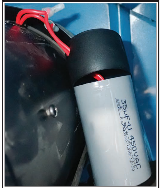
Figure 71. Run Capacitor 35µF 450VAC.
