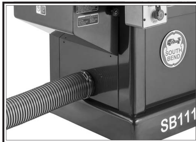
Figure 40. Dust hose attached to port.
