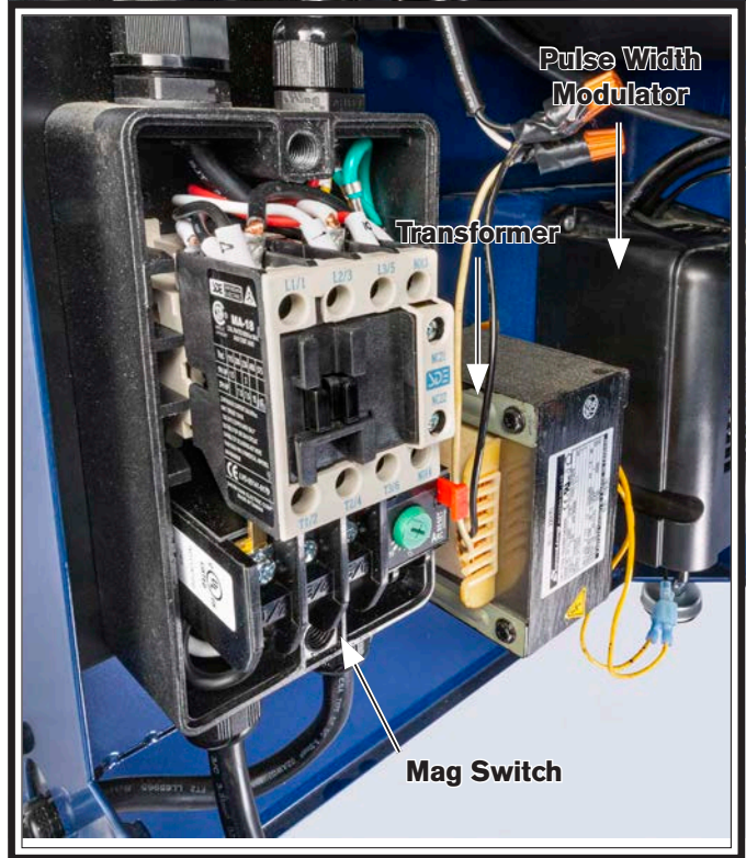
Figure 71. SB1108 mag switch, transformer, & pulse width modulator.
