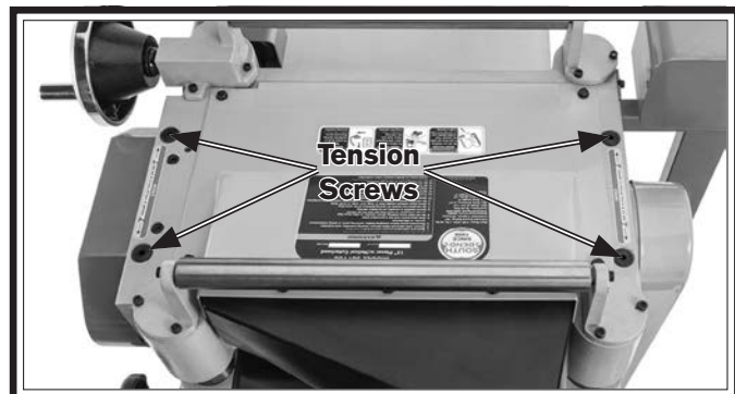
Figure 58. Feed-roller spring tension adjustment screws.
