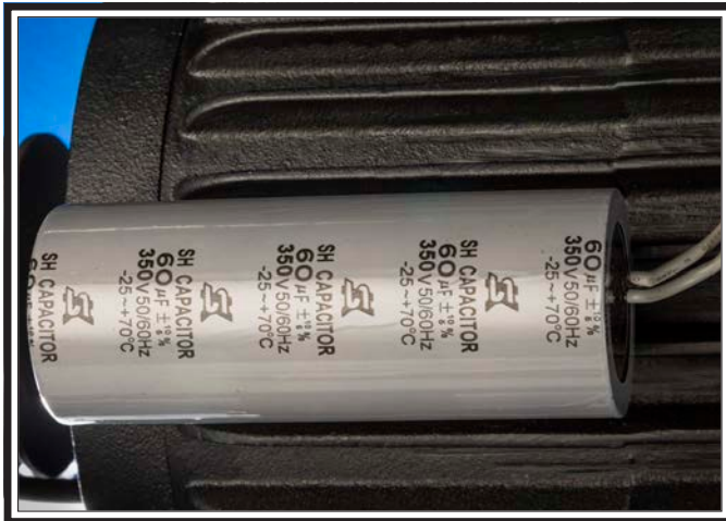
Figure 76. SB1109 run capacitor.
