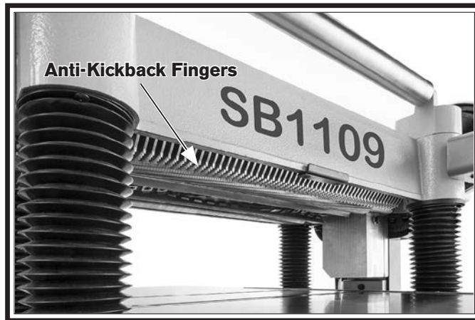
Figure 46. Example of anti-kickback fingers.
