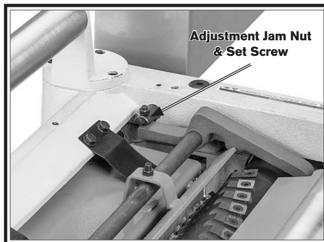
Figure 54. Location of pressure bar height adjustment jam nut and set screw.
