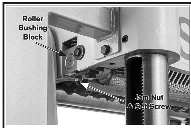
Figure 52. Location of infeed roller bushing block and height adjustment controls (left side shown).
