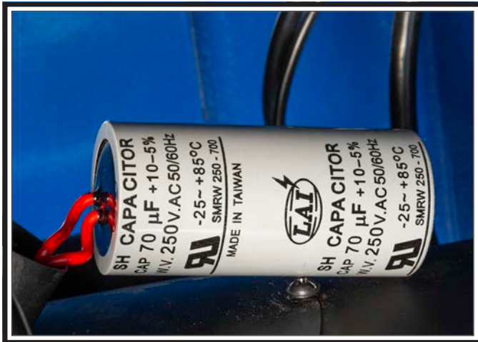
Figure 69. SB1108 run capacitor.
