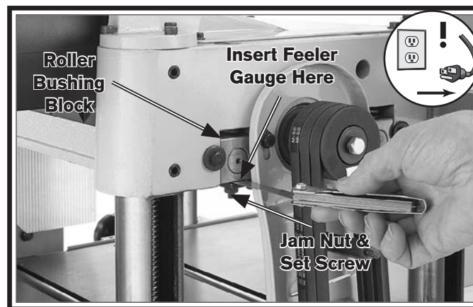
Figure 56. Example of feeler gauge location for adjusting infeed roller height when using wood blocks (one of two locations shown).
