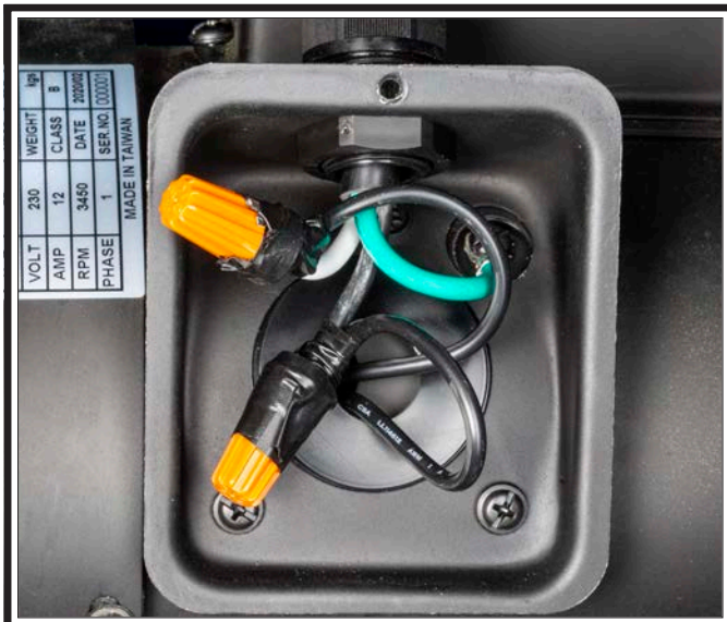
Figure 70. SB1108 motor junction box.
