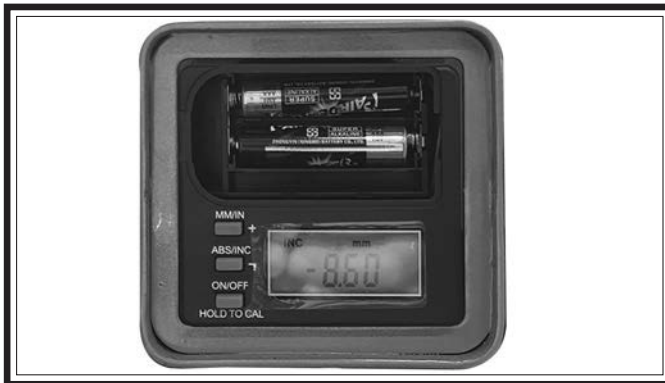
Figure 21. Digital readout batteries installed.
