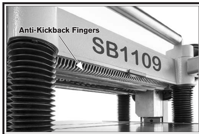
Figure 46. Example of anti-kickback fingers.
