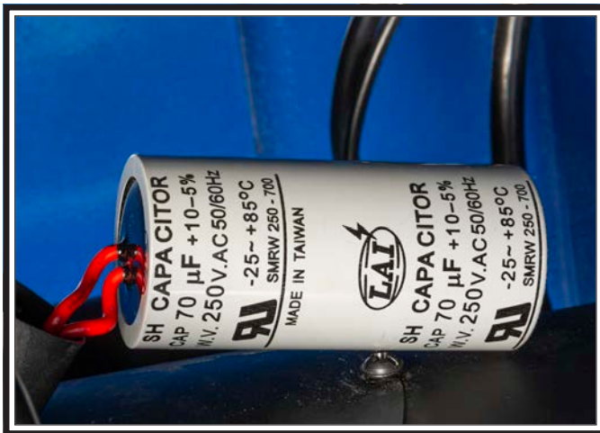
Figure 69. SB1108 run capacitor.
