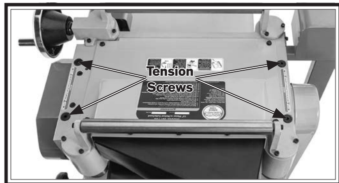
Figure 58. Feed-roller spring tension adjustment screws.
