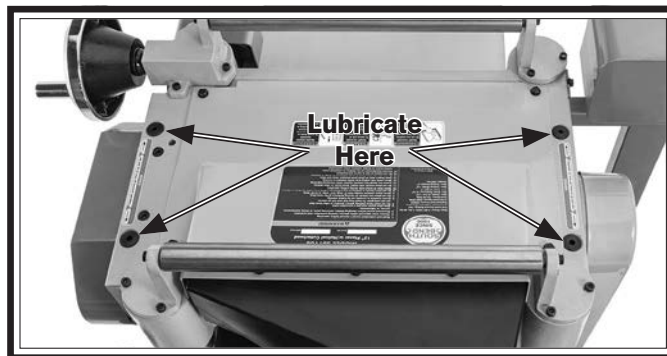
Figure 39. Lubrication locations for feed roller bushings.
