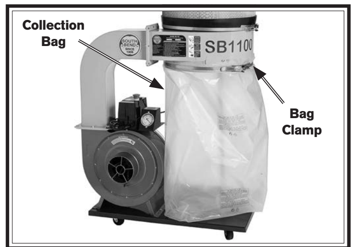
Figure 26. Collection bag installed to dust collector.
