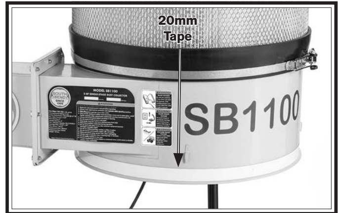
Figure 25. Tape applied to bottom rim of collector.
