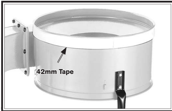
Figure 23. Tape applied to top rim of collector.
