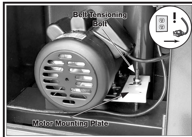
Figure 65. Drive belt tensioning bolt.
