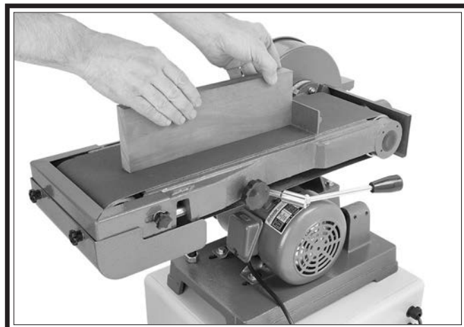
Figure 38. Example of sanding edge of workpiece in horizontal position.
