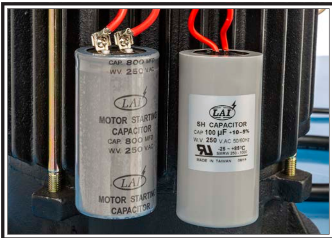
Figure 70. SB1094 capacitor box.
