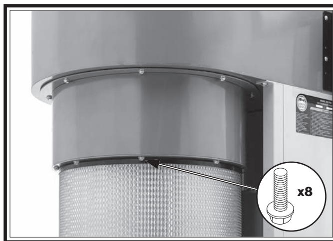
Figure 62. Flange bolts securing canister to housing.
