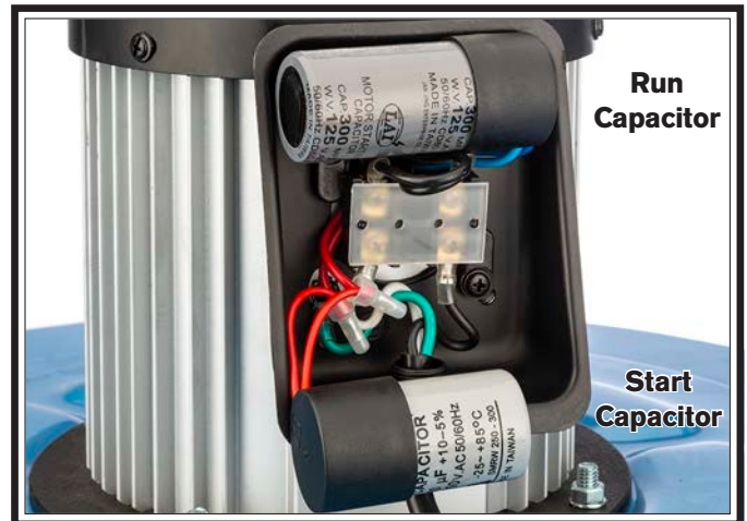
Figure 67. SB1092 main motor junction box.
