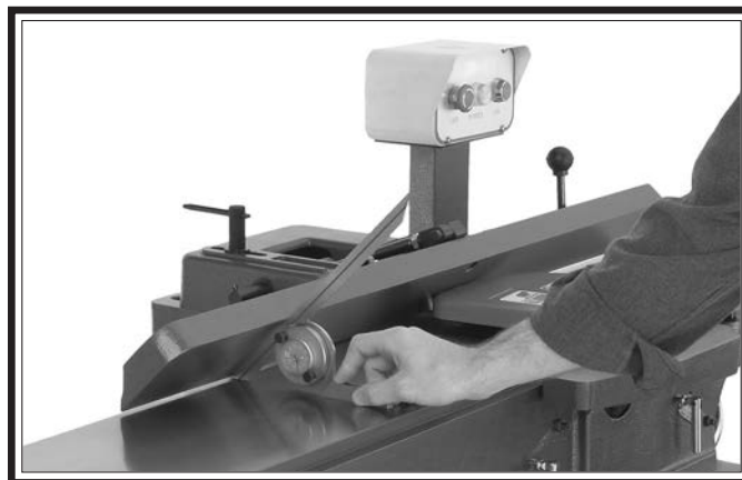
Figure 49. Generic example photo of adjusting fence 45° inward.
