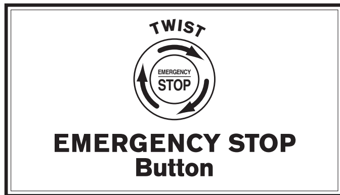
Figure 17. Resetting EMERGENCY STOP button.
