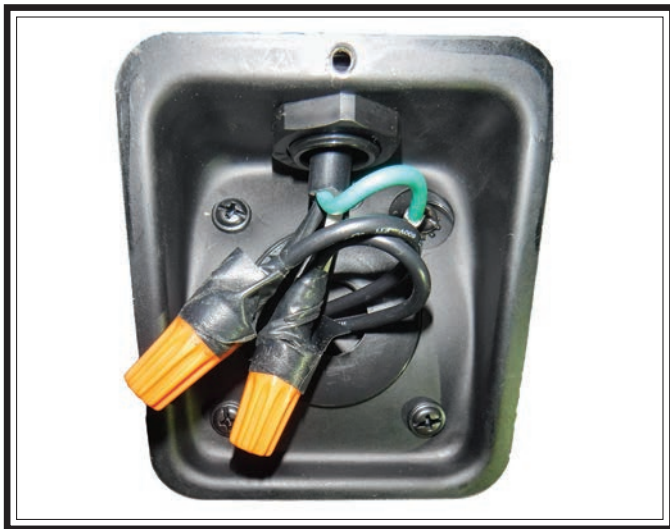
Figure 61. Motor junction box wiring.
