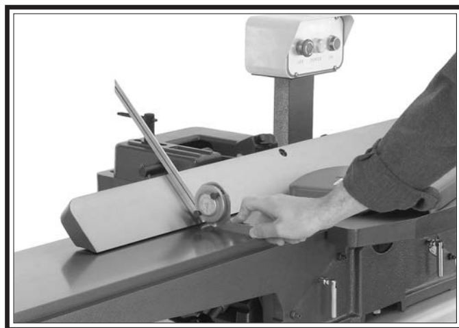
Figure 53. Generic example photo of adjusting fence 45° outward.
