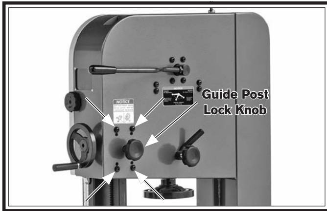
Figure 85. Guide post adjustment screws.
