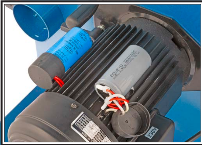
Figure 100. Motor capacitor wiring.
