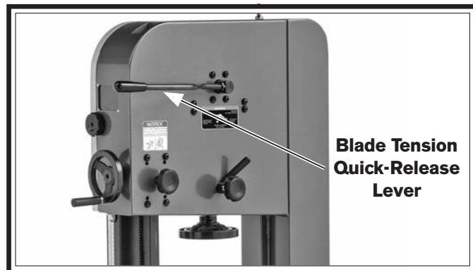
Figure 22. Blade tension quick-release lever in down position, applying tension to blade.
