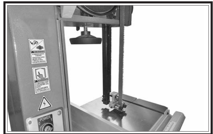
Figure 87. Example of guide post guard removed.
