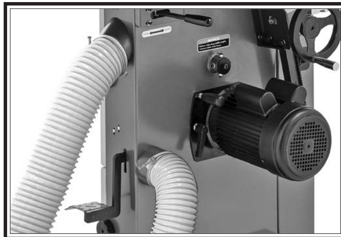
Figure 20. Dust hoses attached.
